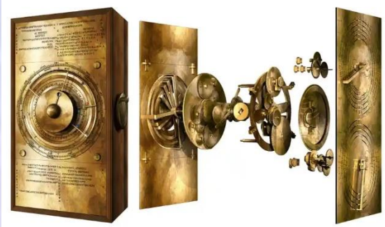
Figure 1: Computer image of the Antikythera Mechanism showing front dial (left), exploded gears and back dials (right).
